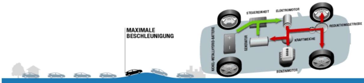
**Abb. 3.2-69:** Toyota Prius, HYBRID SYNERGY DRIVE, Full Acceleration.
